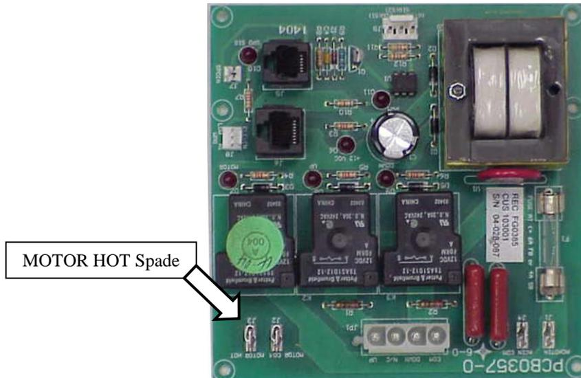
The other end of the inrush limiter will attach to the PWM (motor control) board at the spade marked “L2”. See the diagram below.
