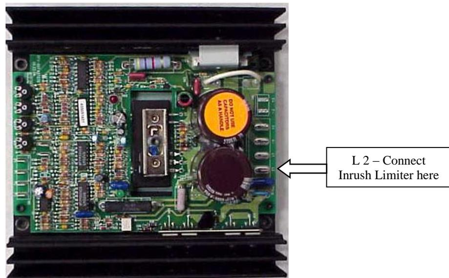
After attaching the inrush limiter to the correct spades, bend the wires of the inrush limiter so that they are out of the way of any fans or moving parts. The black, nickel-sized resistor on the inrush limiter will get very hot while in use, so make sure it does not rest on or touch any other parts under the hood. As always, if you have any questions or problems, please contact the service department at Noramco Fitness.
